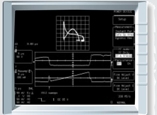
Figures 5A & 5B: Comparison of Safe Operating Area (SOA) measurements before and after channel time-skew correction.
